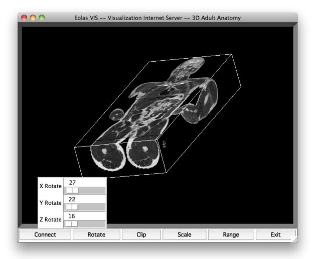
In the above screenshot, the Rotate menu (containing scale widgets for X, Y and Z rotation) is displayed after the user has clicked on the "Rotate" button. Likewise there are scale widgets for Clip, Scale, and the X, Y and Z ranges.
